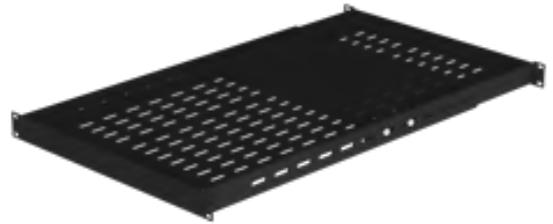
Adjustable shelves with maximum load bearing of 100kg, these versatile shelves adjust to suit rail depths 450mm-750mm & 650mm-950mm.
