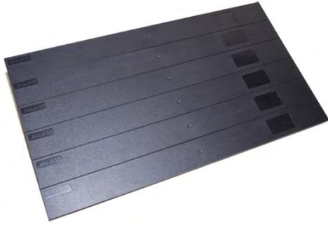
Fitting 19" blanking or EaziBlank panels (and deploying rack air anti-recirculation kits) helps to avoid air mixing and recirculation within the rack space which in turn helps to maximise the cooling infrastructure effectiveness by delivering cool air to the equipment and not allowing it to bypass through empty U spaces.
